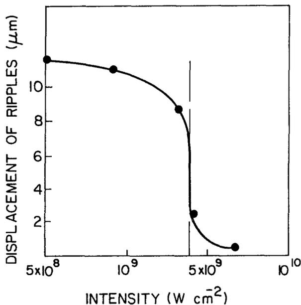
Figure 3 Variation of the inter-ripple distance with the laser beam intensity in the melted irradiated zone.
