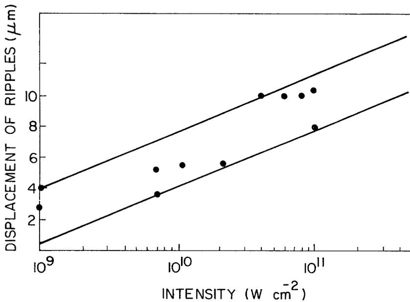
Figure 4 Variation of the inter-ripple distance with the laser beam intensity in the radiation affected zone.
