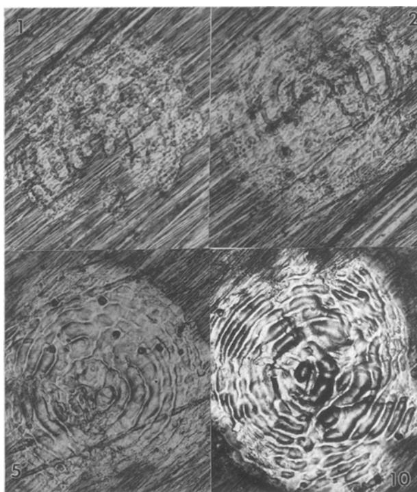
Figure 2 The effect of pulse number on ripples in the melted surface. The number of pulses is shown in each micrograph.
