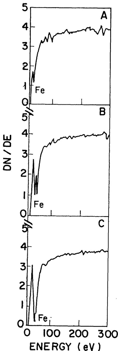
Figure 7 AES analysis of steel irradiated in air atmosphere: (A) surface analysis before sputtering; (B) spectrum of the iron peaks in depth of 120 nm; (C) as (B) but in 300 nm depth.
