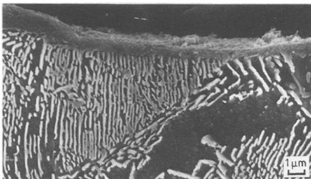
Figure 5 Micrograph showing cross-section of the interaction region of the steel irradiated in air.
