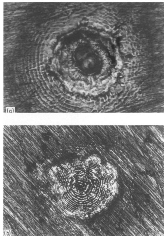
Figure 1 Laser radiation induced ripples (a) in the radiation affected zone (RAZ) and (b) in the irradiation zone (IZ). Magnification  $\times 336$ .
