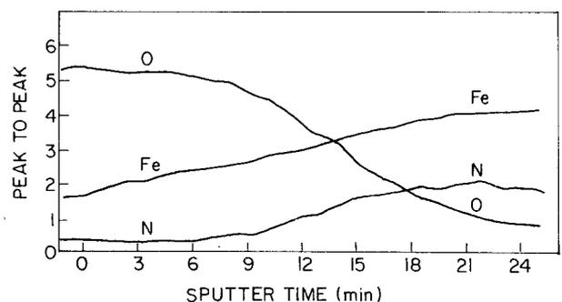
Figure 6 AES depth profile of 1045 steel irradiated in nitrogen atmosphere.
